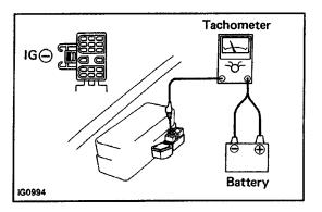
2. With a tachometer is connected to the system, connect the tachometer positive terminal to the IG (-) terminal of the DLC1.
