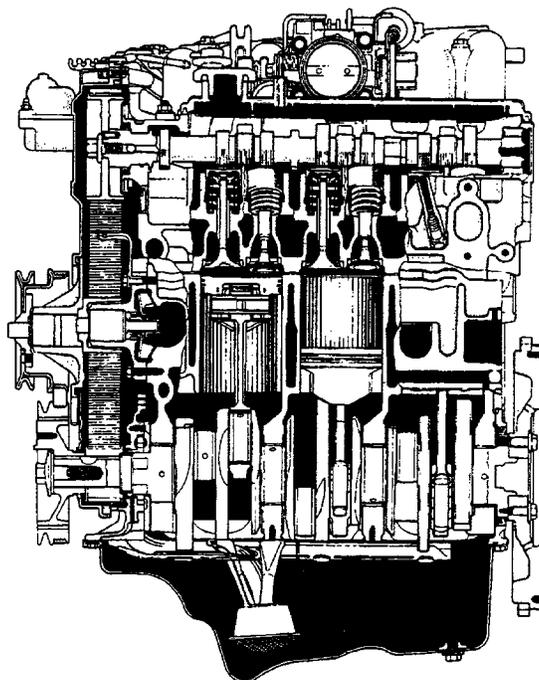
The 3VZ-E engine has 6-cylinders in a V arrangement at a bank angle of 60°. From the front of the right bank the cylinders are numbered 1 – 3 – 5, and from the front of the left bank the cylinders are numbered 2 – 4 – 6.
