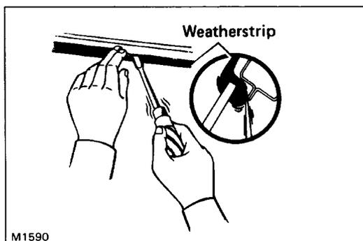
(b) Pry the lip of the weatherstrip outward from the interior part of the body flange.
