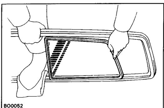
(b) Pull apart the channels and remove two non-slide glass panes as shown.
